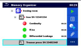
Figure 5.5: Status - Measurements completed with fail result(s)
