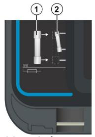
Figure 4.2:Connecting fuses to Fuse checker
