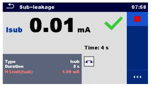
Figure 6.4: Single test screen (during measurement)
