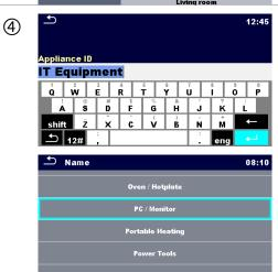
In menu for editing parameters the parameter's value can be selected from a dropdown list or entered via keypad. Refer to chapter 4 Instrument operation for more information about keypad operation.
