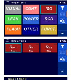
To select another measurement, tap on filed or press the RUN to open menu for selecting measurements. Refer to *Chapters 6.1 Selection* modes and *7.1 Selection of Auto* Sequences for more information.
