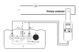
When reading the measured values in V, consider the transformation ratio of the transformer and the fact that the display shows current values as well as the additional display error.
